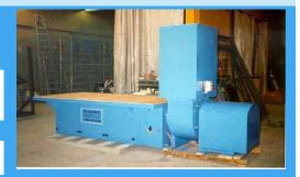
The separate motor/blower assembly has a built in silencer for low noise operation. The spun-bonded polyester cartridge filters are conveniently washable and durable. The finish is medium blue, high gloss machinery paint over primer. Other colours are optional.
